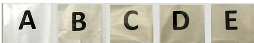
Fig. 2 Photographs of films containing: A neat EVOH 10%; B EVOH/CNC (0.3% wt%)/PdNP (0.3 wt%); C EVOH/CNC (0.6 wt%)/PdNP (0.6 wt%); D EVOH/CNC (1 wt%)/PdNP (1 wt%); E EVOH/TOCNC (1 wt%)/PdNP (1 wt%)
