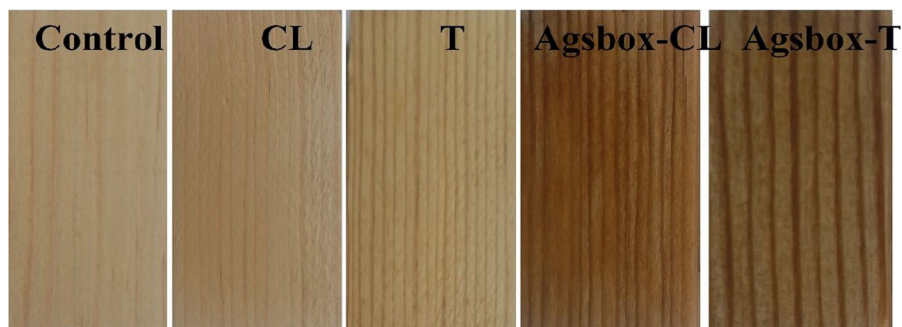
Fig. 2 Colour of treated and untreated specimens ( Control without impregnation, CL impregnated with chloroform, T impregnated with toluene)
