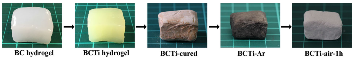
Fig. 2 Photos of BC and BCTi samples. The size of one grid in the background plate is 1 cm × 1 cm
