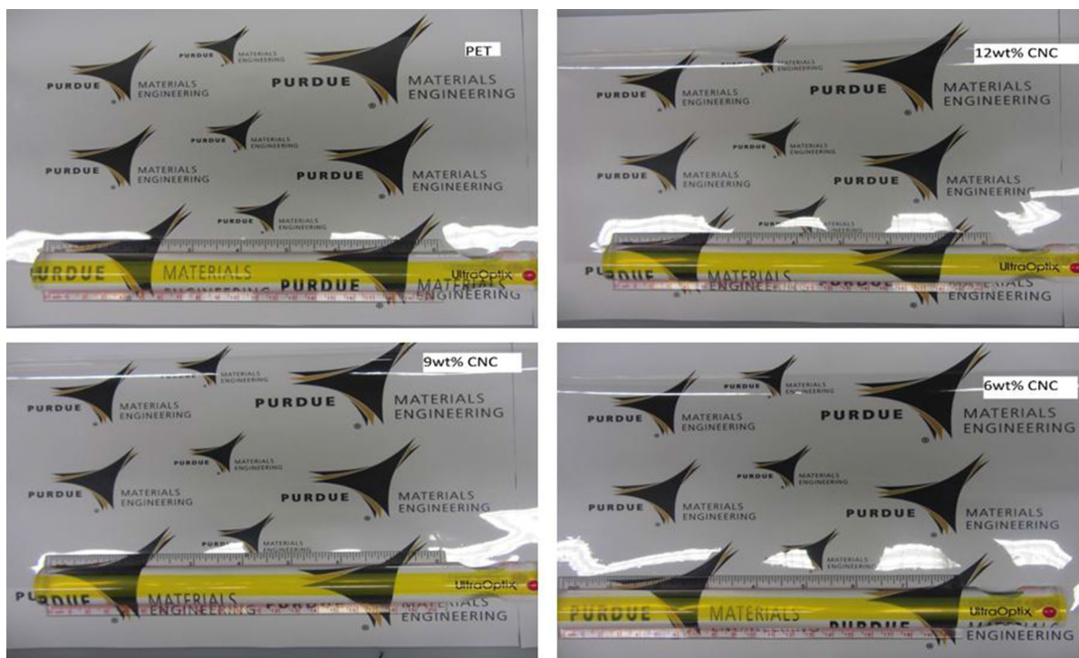
Fig. 8 Photographs of CNC coatings on PET substrate (15 cm × 15 cm): (top left) PET substrate, (top right) 12 wt% CNC solution, (bottom left) 9 wt%, (bottom right) 6 wt%
