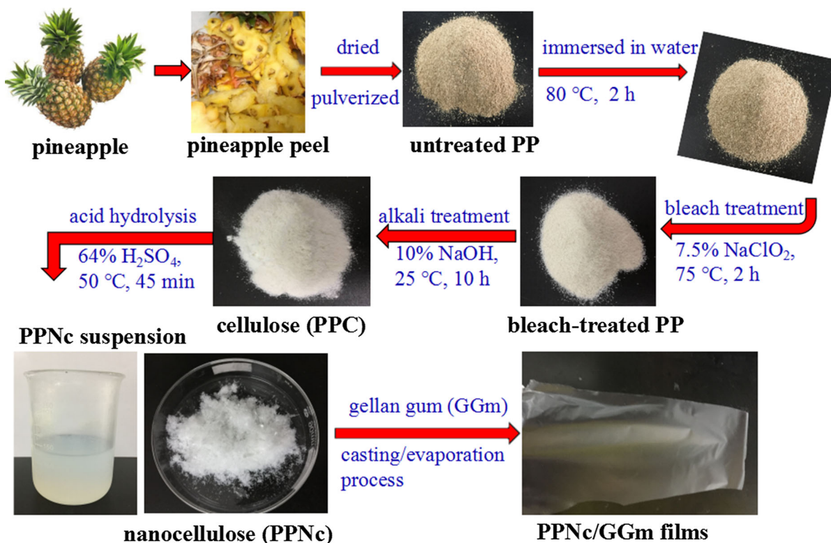
Scheme 1 Experimental procedure for PPnC preparation and its application in GGm films
