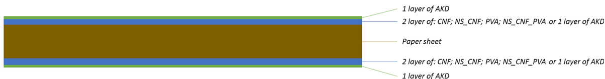
Fig. 1 Schematic illustration of the structure of coated papers
