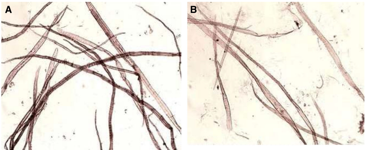
Fig. 11 Unbeaten (a) and beaten (b) pine fibres (optical microscope area, magn. \times 100 ) after being beaten in the Jokro mill for 60 min
