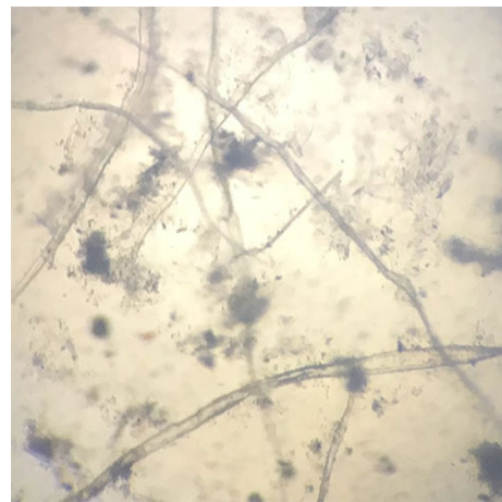
Fig. 7 Ink residue of chemical deinking
