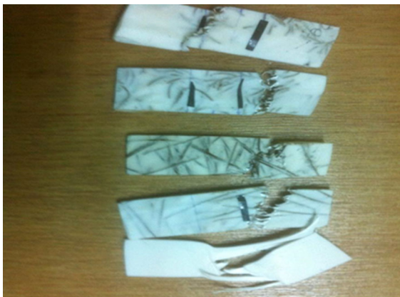
Fig. 3 Broken samples during tensile tests
