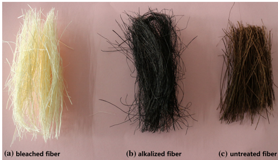
Fig. 1 a Bleached windmill palm fibers, b alkalized palm fibers and c untreated palm fibers
