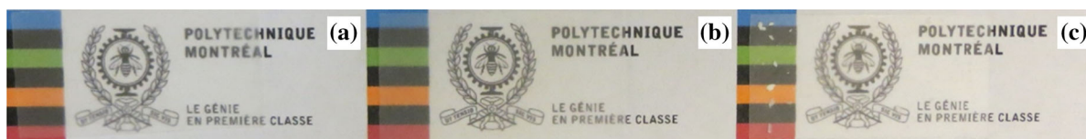
Fig. 10 Visual comparison of a PEO, b PEO/3CNF, and c PEO/3CNF (M) films (thickness of 145 \pm 18 \mu\text{m} )
