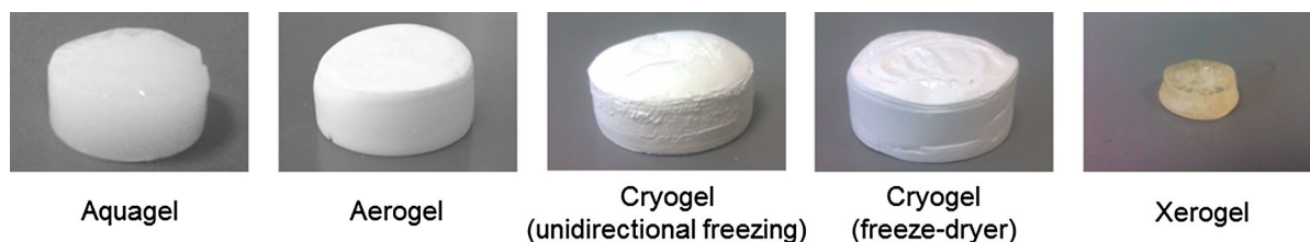
Fig. 1 Examples of an aquagel and samples after drying with different techniques (aerogel, cryogels and xerogel) obtained from 7 wt% cellulose solution
