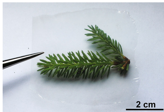
Fig. 1 Regeneration of cellulose/AGX blends from EmimAc results in clear and optically transparent films. The film depicted is a 5 % AGX film
