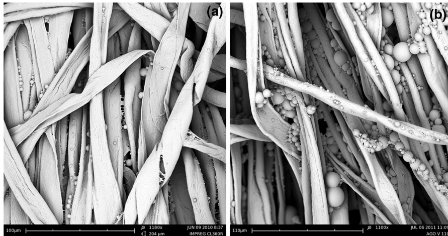
Fig. 1 SEM micrographs of cotton fabrics with microcapsules. a After padding treatment (60 g/L microcapsules and 10 g/L of resin). b After bath exhaustion treatment (240 % owf microcapsules and 40 % owf resin) temperature process 60 °C
