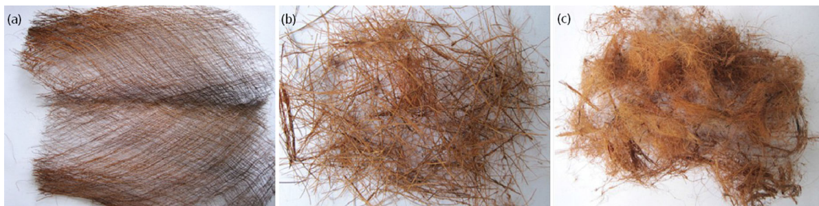
Fig. 1 a The palm-bark; b fibers with larger diameters, longer lengths and more hardness; c fibers with smaller diameters, shorter lengths and less hardness
