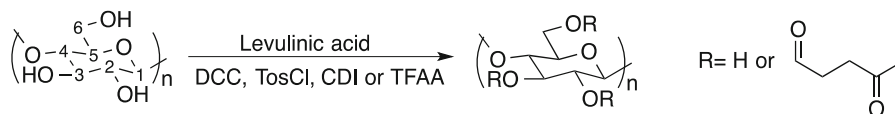
Scheme 2 Reaction of cellulose with levulinic acid and DCC, TosCl, CDI or TFAA in DMAc/LiCl
