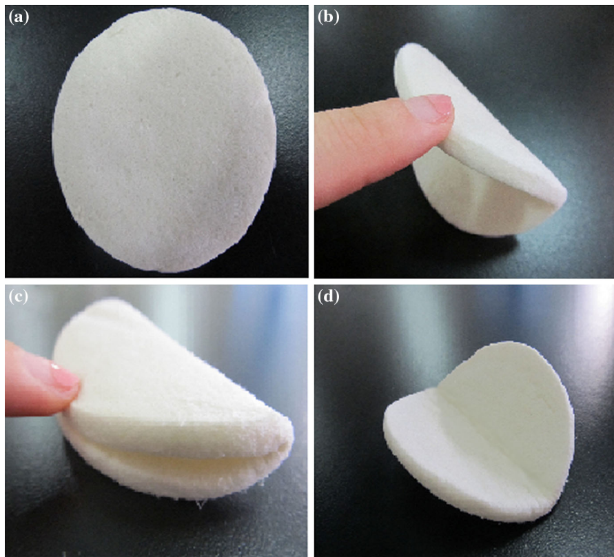
Fig. 4 Morphological images of the chitosan/cellulose composite sponges: (a) flattened sponge, (b) crooked sponge, (c) folded sponge and (d) recovered sponge
