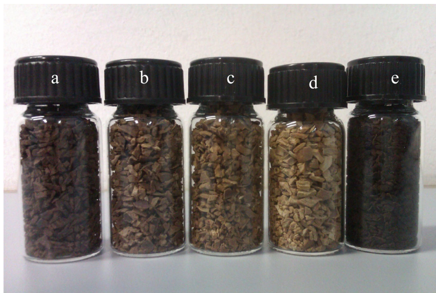
Fig. 2 Pulps after chemical treatment. a Organosolv, b NaOH 15 %, c KOH, d NaOH 7.5 %, e formic acid
