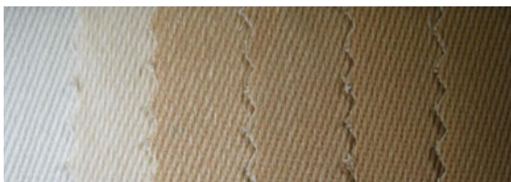
Fig. 5 Image of cotton fabric original and irradiated at various laser fluency (3.1, 4.7, 7.8, 10.9, 15.6 mJ/cm 2 )
