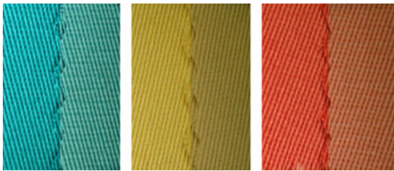
Fig. 7 Image of dyed (1%) cotton fabric original (non-irradiated) and irradiated with the highest laser fluency ( 15.6 \text{ mJ/cm}^2 ) C. I. Vat Green 1, C. I. Vat Yellow 2 and C. I. Vat Red 13
