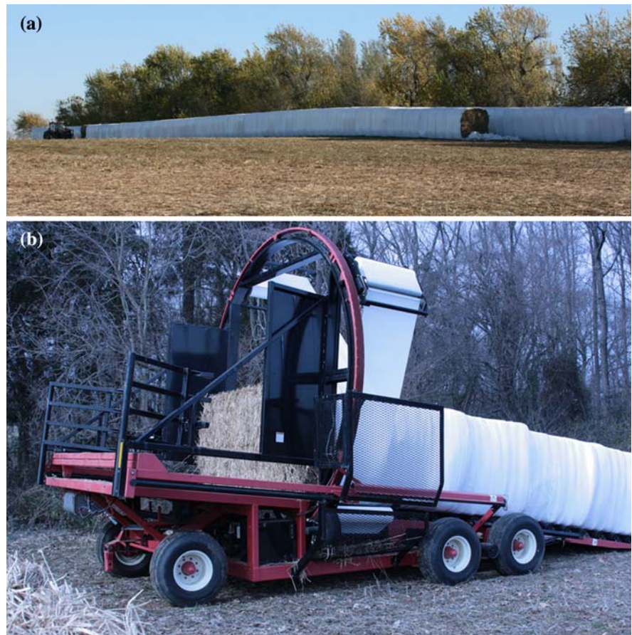
Fig. 4 Plastic-wrapped row of field-side bale stacks (a) that were wrapped with a Stinger 4000 Cube-line wrapper (b)
