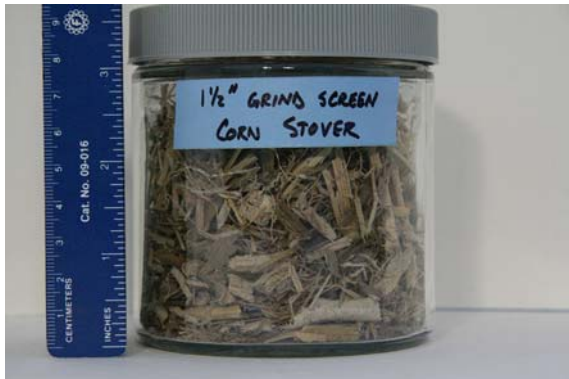
Fig. 9 Corn stover feedstock preprocessed through a nominal 1–1/2 in. minus grinder screen
