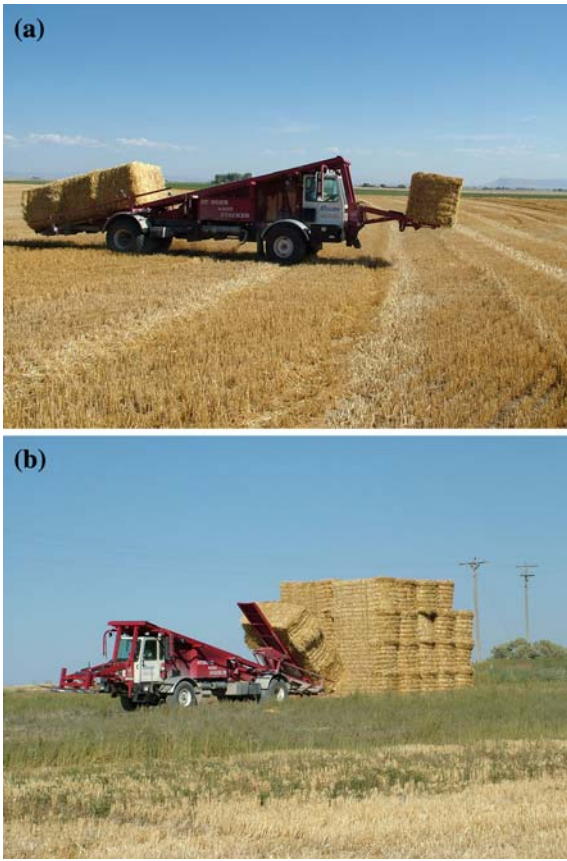
Fig. 3 Stinger Stacker 5500 picking up (a) and stacking bales (b) at bale collection point
