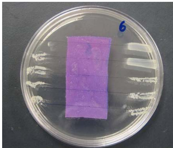
Fig. 3 Antimicrobial property of bamboo viscose fabric treated with 4% reactive dye + 4% Rayosan® + 4% Tinosan®
