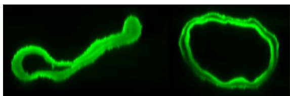
Fig. 4 Radial cross-sections of earlywood fibres saturated with fluorescent labelled polyallylamine (15 kDa) at an ionic strength of 10^{-1} M NaCl for 24 h
