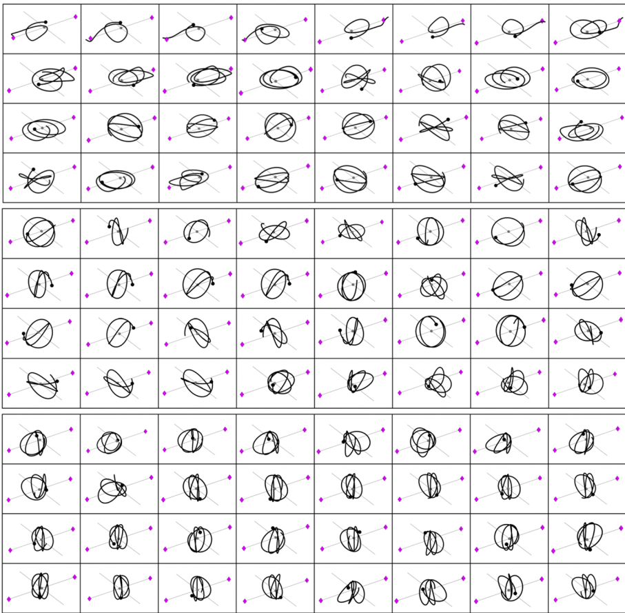
Fig. 13 Subset of representatives for global clustering result summarizing trajectories associated with prograde perigees and generated for up to three returns to a perigee map in the Sun-Earth CR3BP at C_J = 3.00088 , with the libration points displayed as magenta diamonds
