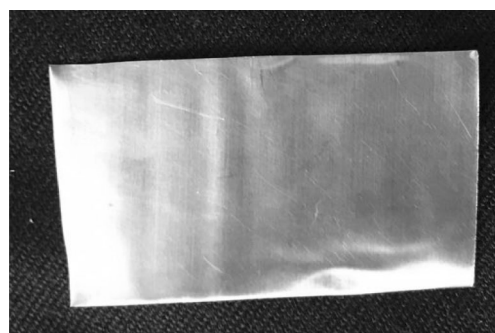
Fig. 1 The image of a sample of deposited silver nanoparticles on commercial copper foil
