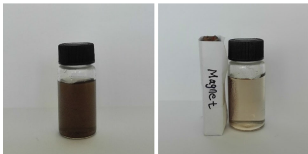
Fig. 4 Magnetic separation of PILs/MCFs
