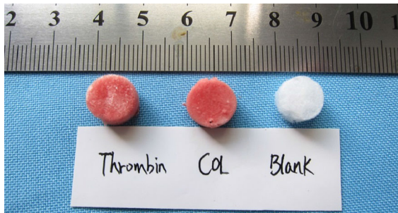
Fig. 1 The COL/PRP scaffolds activated by thrombin or collagen solutions and the blank collagen scaffold
