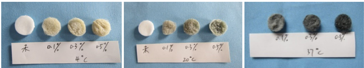
Fig. 2 Collagen scaffolds cross-linked with different genipin concentrations and temperature. The white one is a non-cross-linked scaffold
