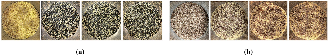
Fig. 1. Exposure of the dispersion composition by the color of the particles being mixed at the time moments of 0, 18, 38, 58 s from the start of the MI operation (initial exposure: (a) colorless particles above, (b) colorless particles below).
