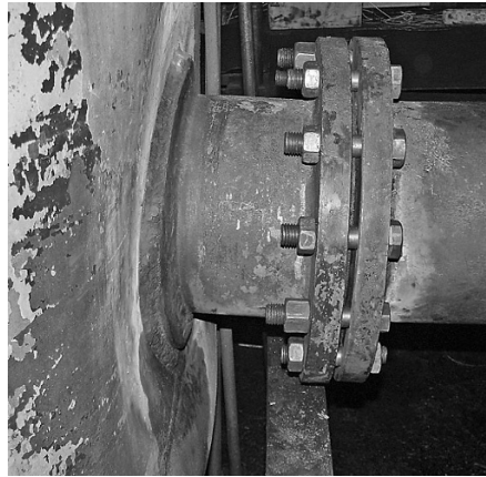
Fig. 2. Depression in region of inlet pipe of filled tank of press.
