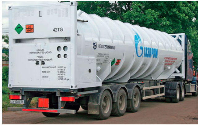
Fig. 1. Cryogenic transporting helium tank TtTG-40/0.45.
