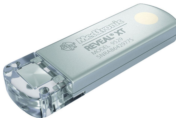
Fig. 1 Reveal XT® ICM. The figure depicts the device used for long-term rhythm monitoring in the study with a dedicated atrial fibrillation algorithm. Reprinted with the permission of Medtronic
