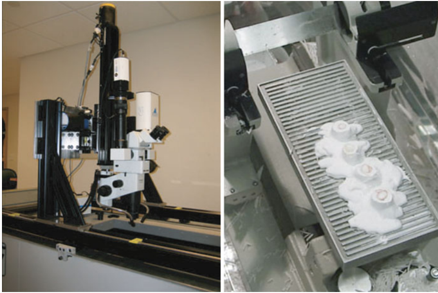
Fig. 5 Cryo-imaging apparatus. Block face images of embedded frozen tissue samples are captured with an episcopic microscope and CCD camera and processed using image processing techniques
