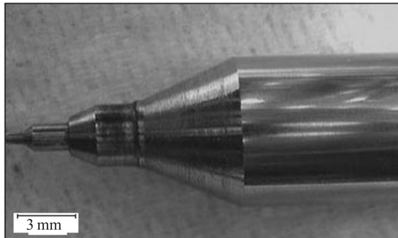
Fig. 1. A micrograph of the injector plunger running on mixed fuel containing 10 vol. % biodiesel.
