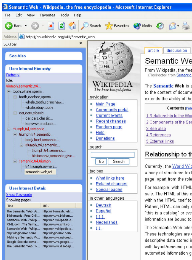
Fig 7 Screenshot, with SEKTbar on the left. At the top, the SEKTbar shows the ontology of the user's interests. Below that, is shown the list of Web pages which correspond to the semantic-web-rdf topic.
