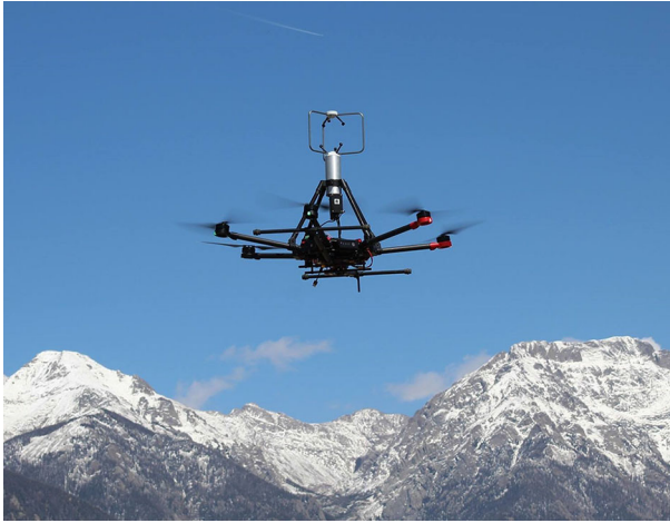
Fig. 4 DJI Matrice 600 hexacopter outfitted with a Young Model 81000 ultrasonic anemometer on top (Photo: Jamey Jacob)
