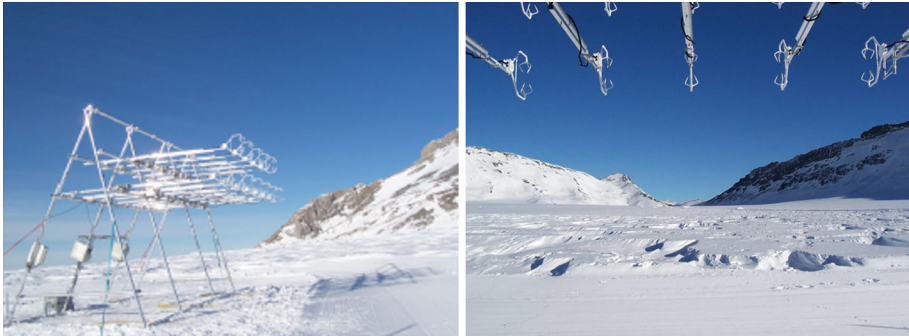
Fig. 1 Set-up of the SnoHATS field campaign. Left: Side view with the 12 instruments. Right: View in the direction of measurements showing the 1500 m fetch
