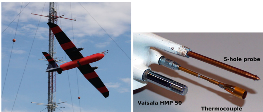
Fig. 3 The M 2 AV flying past the meteorological tower at MOL-RAO and its sensor dome
