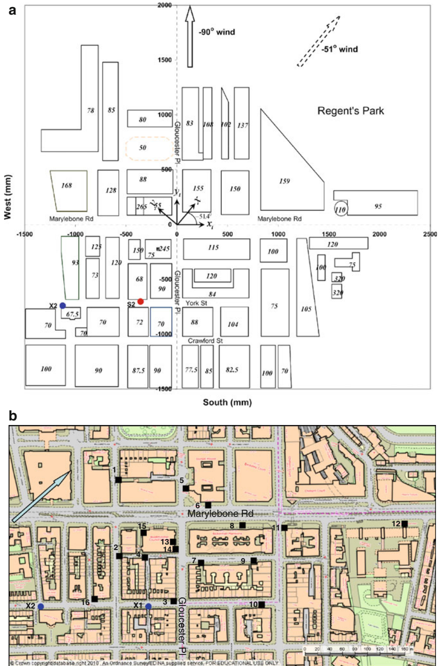
Fig. 1 Plan view of the DAPPLE site. a 1:200 WTM: numbers in italics on each building block indicate its height in mm; the model coordinates are marked in mm, with x_t from west to east, y_t from south to north and z from ground to top respectively; x , y , z are the computational coordinates (Fig. 2). b Full-scale field experiment site: X1, X2, source sites; square symbols, sampling sites. The base map is an Ordnance Survey/EDINA supplied service (© Crown copyright / database right 2010)
