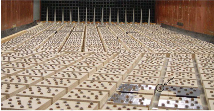
Fig. 1 Wind-tunnel experimental set-up and source position
