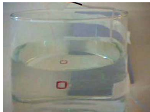
Fig. 9 Picture of an elastic polymer tail in a container filled with water and placed at the homogeneous region of the MRI
