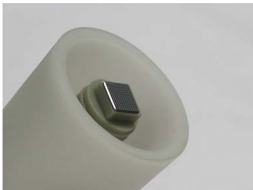
Fig. 8 The head of a microneedle intradermal drug delivery system. The microneedle array was fixed onto the supporting column of the applicator, which had a retainer ring
