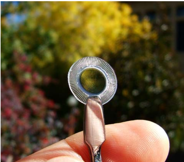
Fig. 10 A photolithographically patterned artificial cornea prototype with central optic and peripheral skirt. The central optic is composed of a PEG/PAA double-network hydrogel, which is interpenetrated in its periphery with a microperforated PHEA hydrogel skirt
