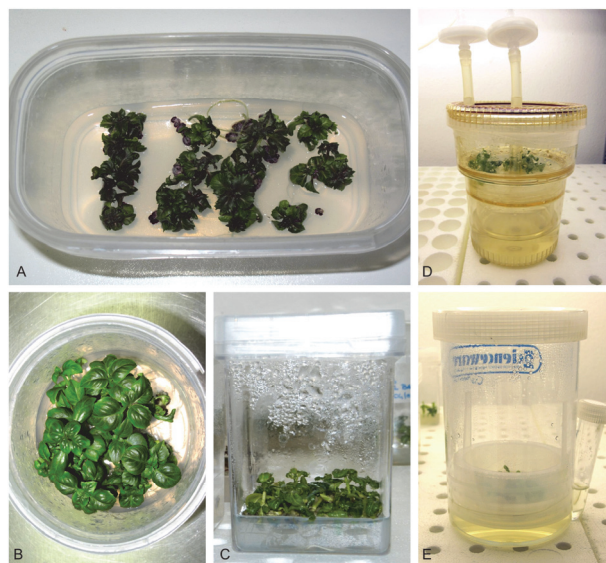
Fig. 1. Types of vessels used for the in vitro culture of sweet basil shoots: A - Microbox ECO 2 TM , B - PCCV25 TM , C - GA-7 box Magenta TM , D - temporary immersion system RITA TM , E - cylindrical bioreactor Growtek TM .
