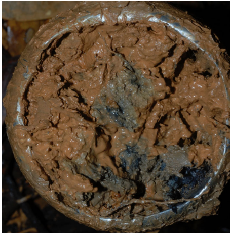
Fig. 2 Cross-sectional photo of the bottom of a soil core (6 cm diameter, 0–10 cm depth) collected from a slope position in the Luquillo Experimental Forest. The pronounced gleyed regions at the center and bottom of the image, present within a ferric orange matrix, visually illustrate the spatial heterogeneity of reduced and oxidized Fe within surface soils in this ecosystem
