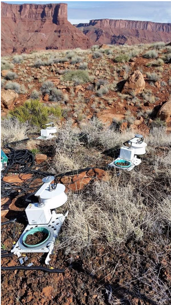
Fig. 1 The research site along with three LI-8100-104 opaque automated soil CO 2 flux chambers. Each chamber was installed in biocrusted interspaces >5 cm from the nearest perennial grass or shrub canopy. During installation, rock walkways were installed to allow access to each chamber while minimizing repeated soil surface disturbance near the chamber because of concerns about minimizing dust production
