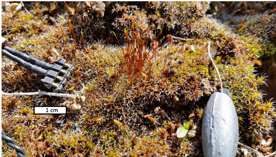
Fig. 3 Surface moisture ( left ) and temperature ( right ), installed in Syntrichia caninervis biocrust
