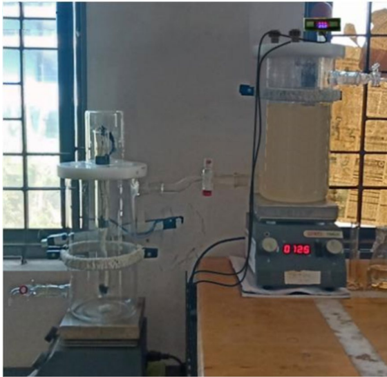
Fig. 2 Photographic view of the batch reactor showing degradation experiments using free cells of P. aeruginosa STV1713
