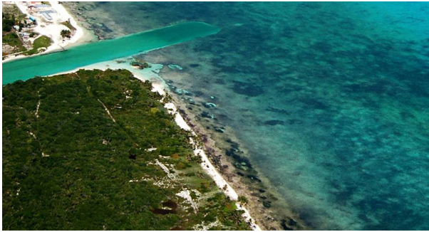
Fig. 4 The opening of the Zaragoza canal into the reef lagoon at the southern Mexican Caribbean. The area was levelled by using dynamite. Photograph, Humberto Bahena
