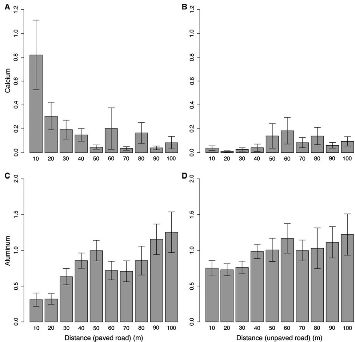
**Fig. 2** Calcium rates ( $\text{cmol}/\text{dm}^3$ ) and Aluminum rates ( $\text{cmol}/\text{dm}^3$ ) along a gradient of 100 m from the paved road and unpaved road. High content of calcium at the roadside in
