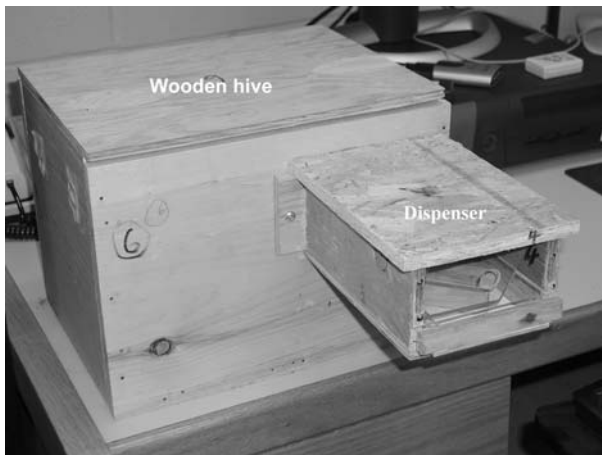
Fig. 1 Wooden dispenser (21 × 12 × 8.5 cm) affixed to wooden hive (32 × 23 × 24 cm)
