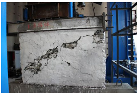
(a) Oblique cracks
